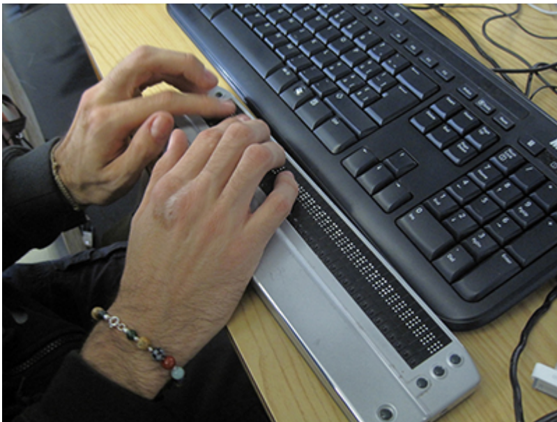
Refreshable Braille device being used. Photo from Flickr by Visualpun.ch.
